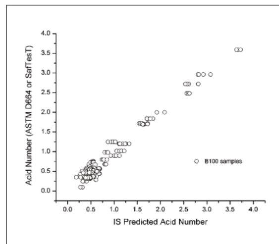
Figure 7. Acid Number D664 versus IS Predicted Acid Number
