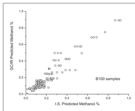
Figure 6. GC/IR versus IS Estimated Methanol Concentration - B100
